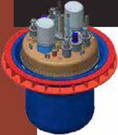
Fig. 5.2: The layout of the MYRRHA reactor vessel.
