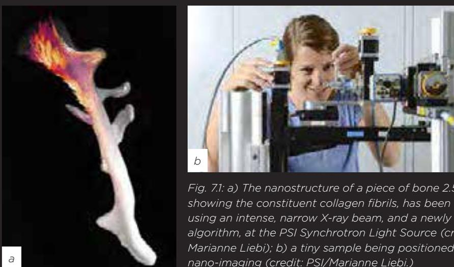
Fig. 7.1: a) The nanostructure of a piece of bone 2.5 mm long, showing the constituent collagen fibrils, has been mapped using an intense, narrow X-ray beam, and a newly developed algorithm, at the PSI Synchrotron Light Source (credit: PSI/Marianne Liebi); b) a tiny sample being positioned for 3D nano-imaging (credit: PSI/Marianne Liebi.)
