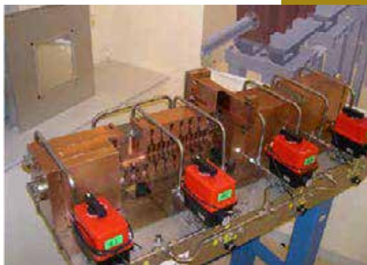
*Fig. 3.8: The TERA side-coupled linac structures (shown) and other, later high-gradient structures have been proposed for a variety of particle-therapy applications, including proton and carbon-ion treatment, and the delivery of very high-energy protons for imaging and novel treatments (credit: Adriano Garonna/TERA Foundation).*
