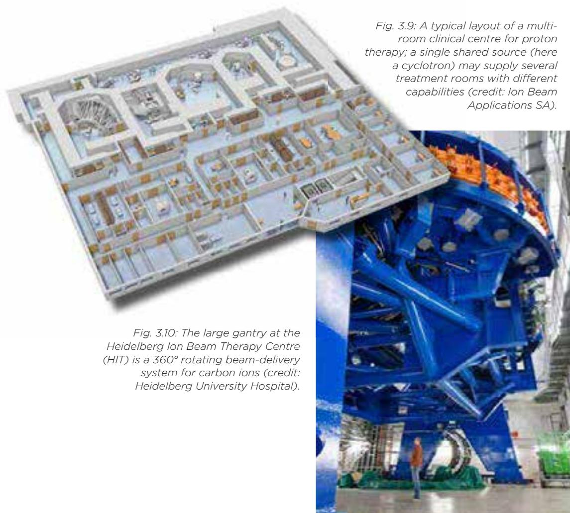
*Fig. 3.10: The large gantry at the Heidelberg Ion Beam Therapy Centre (HIT) is a 360° rotating beam-delivery system for carbon ions (credit: Heidelberg University Hospital).*
