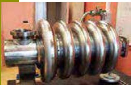
Fig. 2.7: Superconducting accelerating cavities (credit: CEA).
