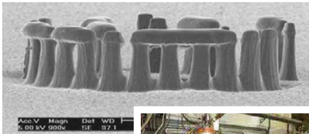
*Fig. 4.26: In this micro-machined Stonehenge-like structure, which is 80 micrometres in diameter, the horizontal 'stones' are fabricated by a beam of 500-keV protons (range in silicon about 6 micrometres) and the vertical 'stones' by 2-MeV protons (range about 48 micrometres). (Reproduced from F. Watt et al., Materials Today, 2007, **10**, 20.)*
