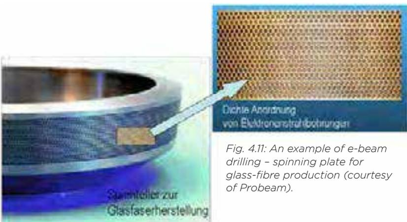
Fig. 4.11: An example of e-beam drilling - spinning plate for glass-fibre production (courtesy of Probeam).
