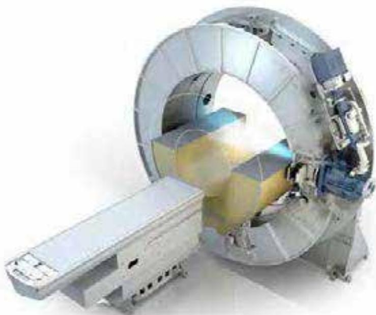
*Fig. 3.4: The MR-linac, developed by Elekta, consists of a linear accelerator equipped with multi-leaf collimator technology for accurate radiotherapy dosage, combined with a high-field MR imaging system. The MR-linac is work in progress and is not available for sale or distribution (courtesy of Elekta).*
