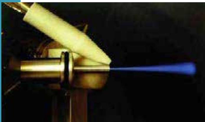
Fig. 4.18: A 3-MeV proton beam extracted into air.
